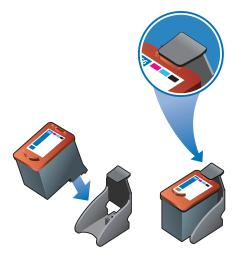
2 To remove the print cartridge from the protector, press down and back on the tab inside the protector to release the print cartridge, and then remove the print cartridge.
